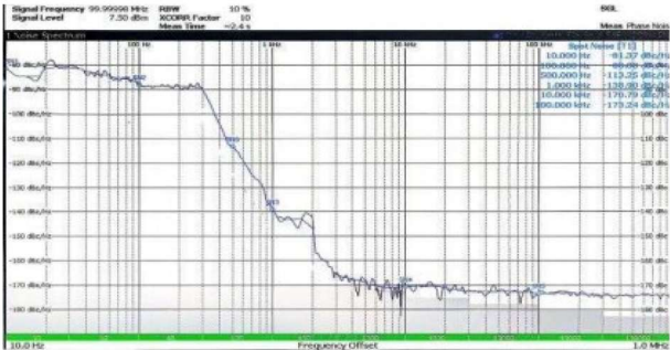
Typical dynamic phase noise curve for a 100 MHz crystal oscillator 1,000 MHz crystal vibration spectrum line graph
