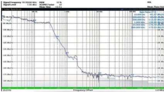
Typical dynamic phase noise curve for a 100 MHz crystal oscillator 1,000 MHz crystal vibration spectrum line graph
