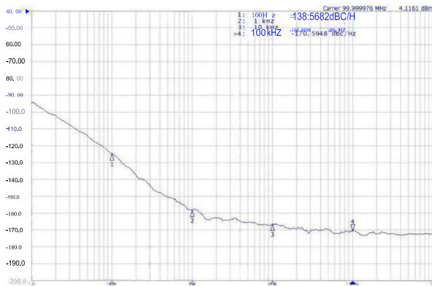
100 Typical phase noise curve of an MHz crystal oscillator
