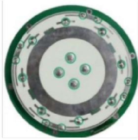
Antenna dimensions: \phi 127.8 \times 20.3 mm
