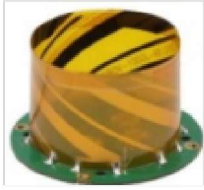
Antenna dimensions: \phi 44 \times 28 \text{mm}
