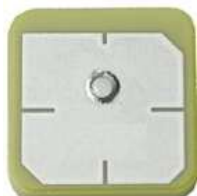
Antenna dimensions: 18*18*4 mm
